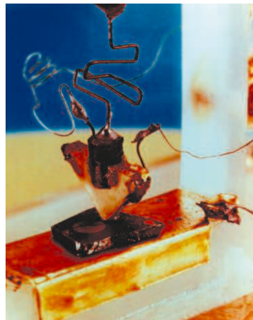
The first transistor (1947). To obtain power gains, Walter Brattain had to reduce the separation of the two metal point contacts on the germanium crystal to under 50 \mu\text{m} .
